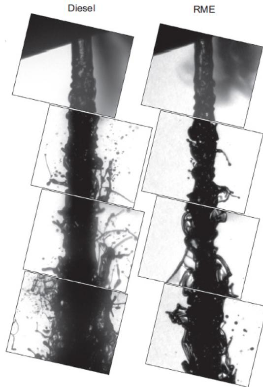
Figure 1. Influence of fuel type on the primary atomisation within the first 2.1 mm from the nozzle (left is diesel fuel and right is biodiesel (RME)).
